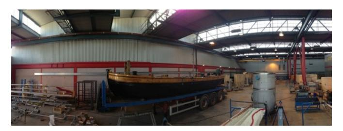
The trow team indeed rolled up their sleeves, both this month and in October last year, and got stuck into d.i.y. maintenance. Every inch has been washed and scrubbed. Nielsen's have re-caulked the decks and repaired a small area of underwater damage to the hull. The hull and bilges have been repainted with bitumen. All the rest of the woodwork has been re-treated with different grades of deck oil. THB is now gleaming.
